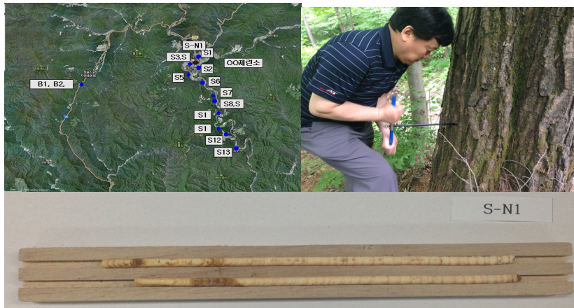
<Figure 5> Sampling of wood core (A) The map of samplein site nearby zinc refinery (B) The method of wood core sampling (C) An example of wood core samples.
